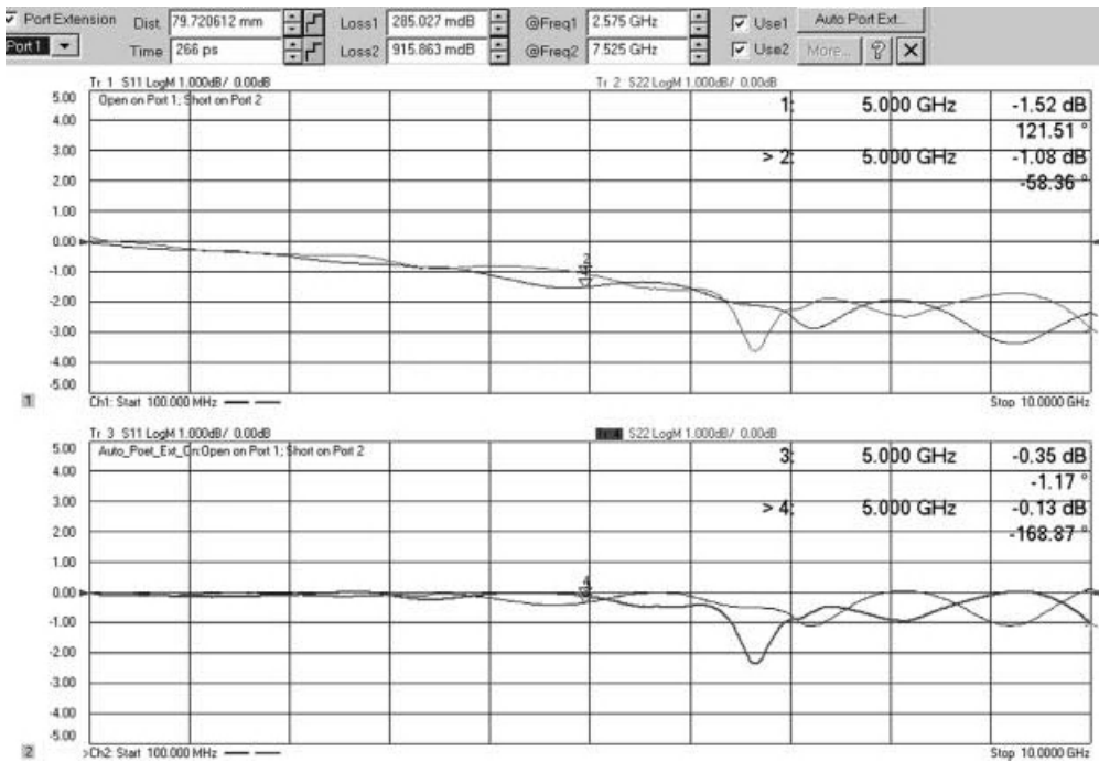
Figure 9.21 (upper) Measurement of an open and shorted fixture; (lower) after automatic port extensions.
