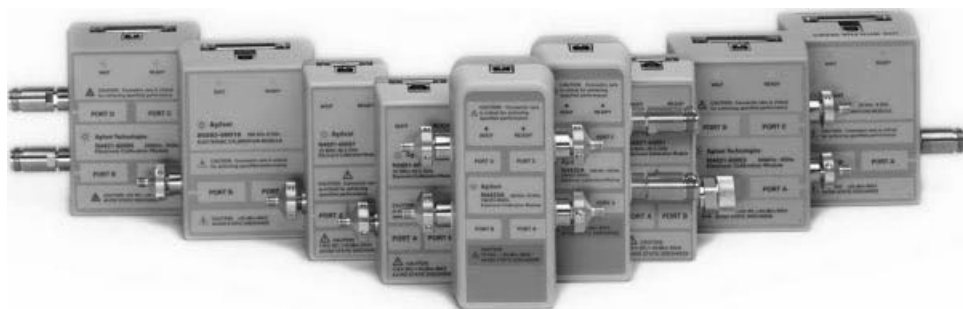
Figure 3.17 Ecal modules are available in a variety of port configurations, connectors and frequencies. Reproduced by permission of Agilent Technologies.
