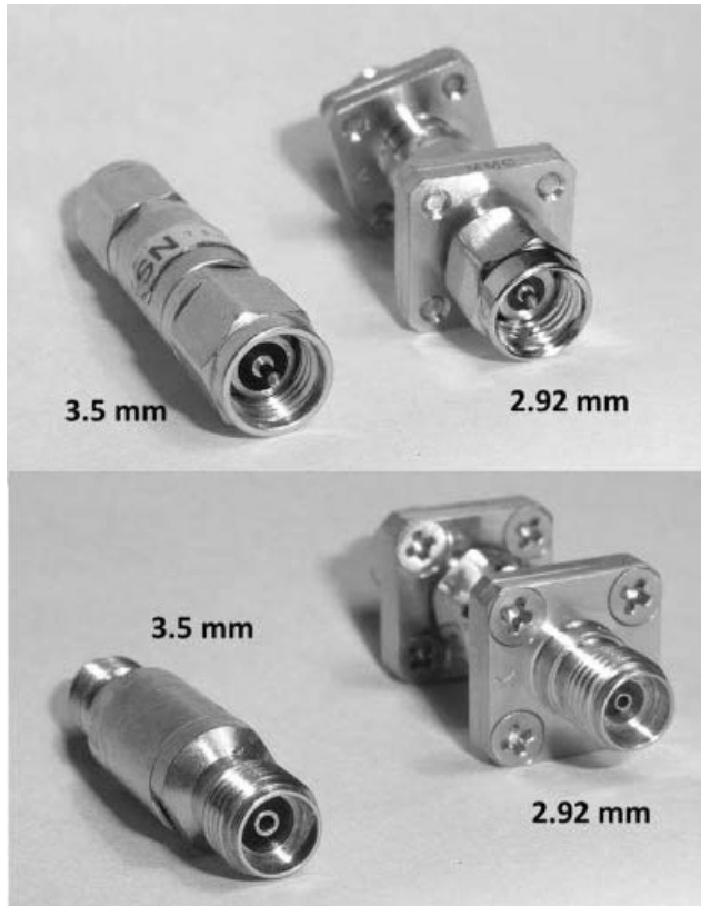
Figure 1.23 A 3.5 mm connector (right) compared with 2.92 mm, male and female.
