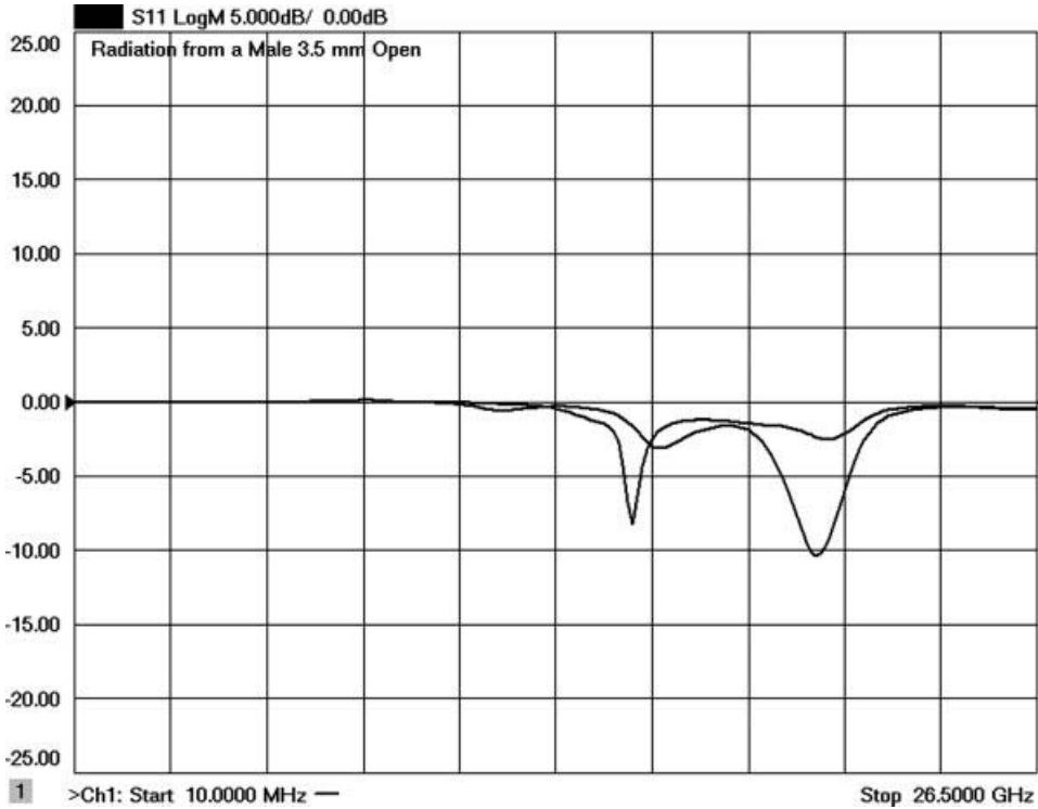
Figure 3.8 Variations in the open reflection coefficient due to radiation for an unshielded male SMA.
