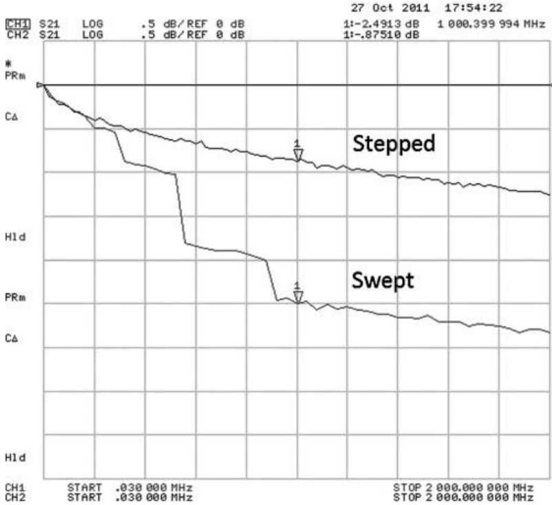
Figure 5.4 Comparing stepped with swept mode on a 3 m cable insertion loss measurement.
