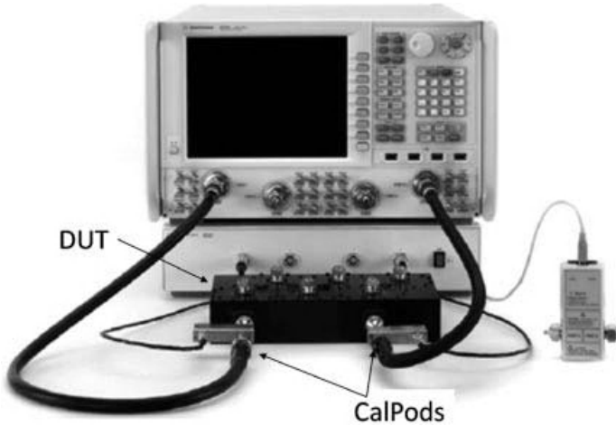
Figure 5.16 Example of a re-correction system for removing test cable drift. Reproduced by permission of Agilent Technologies.
